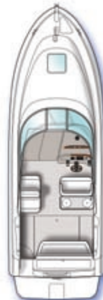
COCKPIT LAYOUT W/STANDARD SEATING (Shown w/Optional Bait-Prep Station)
